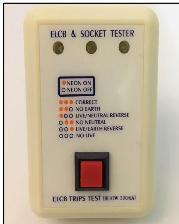
Rajah 5: Penguji Soket ( Socket Tester )
