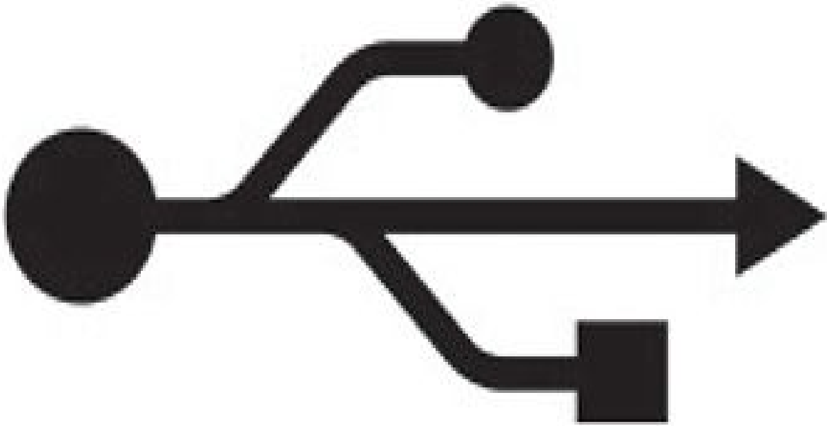
FIGURE 11-9 The ubiquitous USB logo, indicating a port that will accept a USB cable connector.
