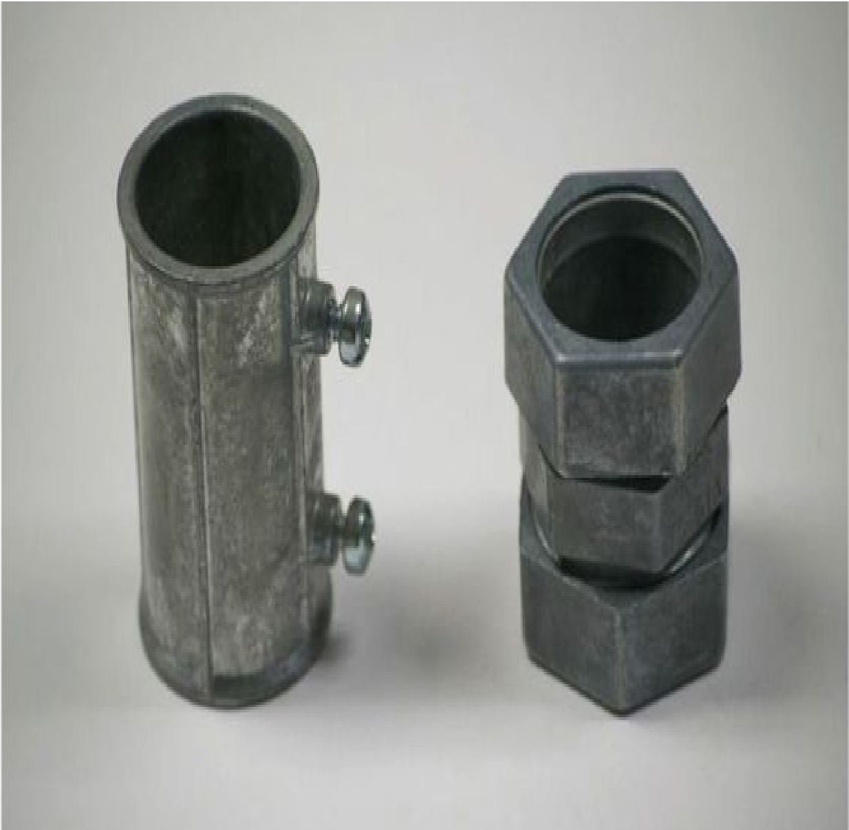
FIGURE G-15 Type EMT fittings: set-screw type at the left for indoor work and compression-type at the right for outdoor work.
