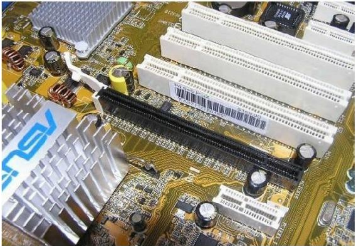
THE PCI-EXPRESS GRAPHICS CARD SLOT ON THE MOTHERBOARD
